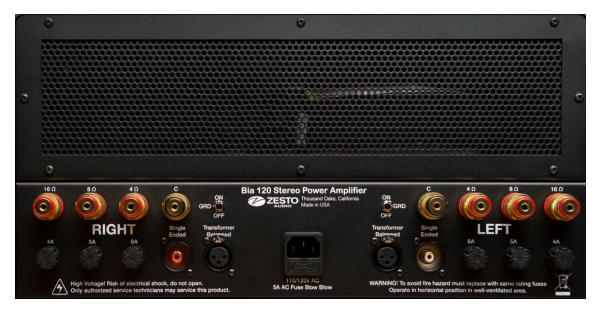
Power ON/OFF switch ......Turns the unit ON/OFF (located on front panel). Amber indicates low voltage (Both lights will remain on when unit is in use) Fuse installed in mains inlet connector. Optional factory installed 220V, 230V/240V mains with 3.15 Amp slow blow fuse. gold pin connectors to the Balanced inputs Outputs Left and Right....... 5 way binding posts with 4, 8 and 16 Ohm taps with Black common for each output tap
